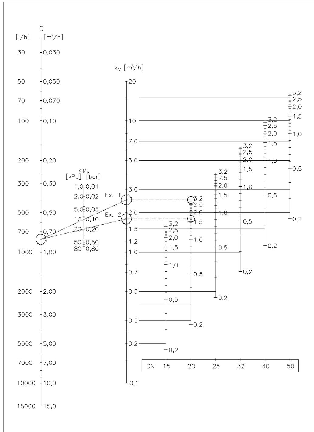
A straight line connecting the bars of flow, differential pressure and  $k_v$  value shows the relationship between these three variables.
