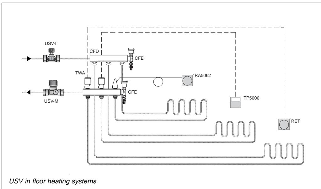
Upgradable control valves are to be used for manual balancing of a floor system manifold.
