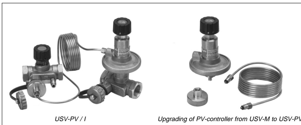
USV-PV (blue knob) is designed to maintain a constant set differential pressure across a riser. Eventual operating noise caused by high differential pressure induced by changes in the system can be avoided by upgrading the manual valve to the differential pressure controller.
