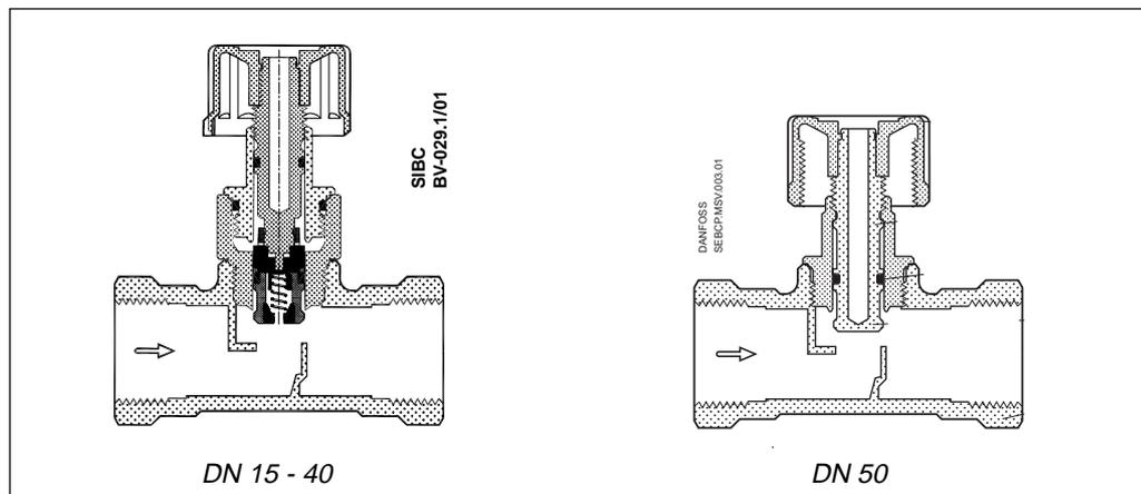
USV-M can be upgraded to USV-PV automatic balancing valve. The system does not need to be depressurized during the upgrade.
