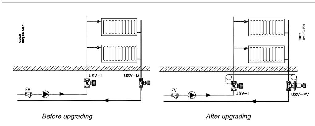
Upgradable USV valves are to be used for manual as well as automatic balancing of heating systems. If system has to be fitted with differential pressure controller, USV can be upgraded with PV controller.
