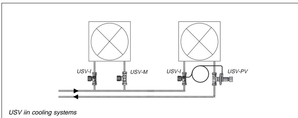
Upgradable USV control valves are to be used for manual or automatic hydronic balancing of cooling devices i.e. as fan coils or chilled ceilings.
